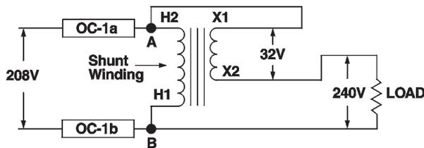
*Overcurrent devices OC-1a and OC-1b are shown correctly installed in accordance with 450-4. Locating an overcurrent device in series with the shunt winding anywhere between A and B is not permitted. The shunt winding is the winding common to both the input and the output circuits.*
